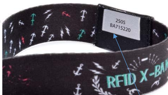
Embedded RFID tag in woven pouch Printed UID & serial number
