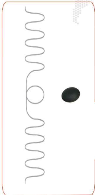
Textile laundry tag consists of 3 main parts which can withstand harsh industrial environment for laundry processes operating for hundreds cycles.
